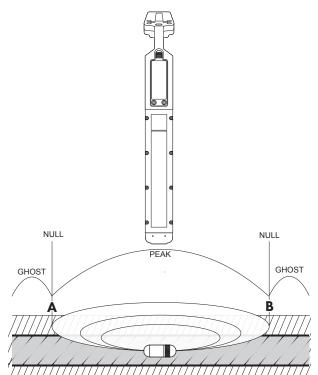
DISTANCE BETWEEN A AND B TIMES 0.7 EQUALS DEPTH OF SONDE.
