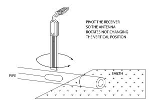
Now move the Receiver side to side (across the path of the pipe) as shown below. When the PEAK if found, the Receiver is directly over the Sonde. Mark this location. Next, check for ghost signals in front of and in back of the Sonde to confirm the location.
