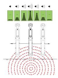
If you rotate the RECEIVER while over the cable, a sharp NULL will identify the cable's direction. It is aligned with the flat side of the RECEIVER.
