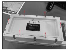
Remove the Li-Ion tray's screws
